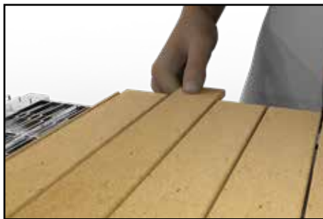
Sectional stone belt with individual stones easily replaced if necessary. The holder for an individual stone is released, enabling the easy removal of the stone from the side.
