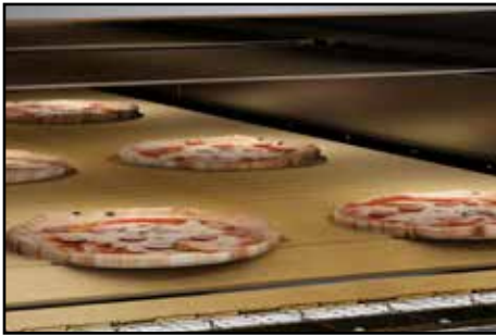
The stone hearth belt for baking pizza, flatbread, pita bread, naan bread, etc.
