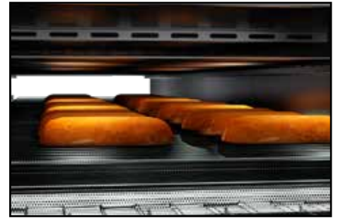
The perforated steel belt is used for free-form, high-rise loaves and the like.
