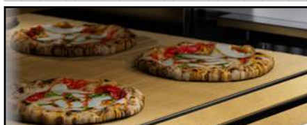
The stone hearth belt for baking pizza, flatbread, pita bread, naan bread, etc.
