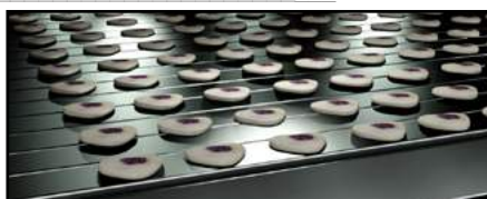
The steel belt is used for sweeter doughs and low-rise products such as cookies.
